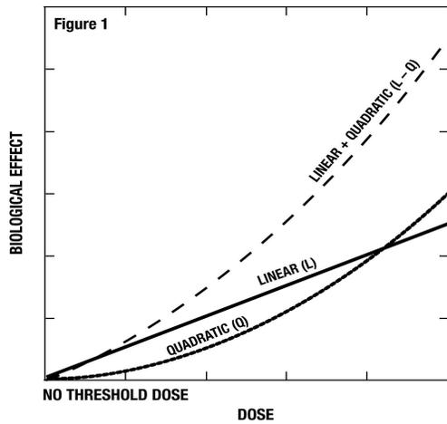
Figure 1. The relationship between biological effect and dose. The linear quadratic effects are combined to show the total effect described by the Linear + Quadratic (L-Q) curve. There is no threshold dose (the Linear No Threshold model).
