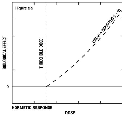
Figure 2a. A threshold dose applies which indicates there is no biological effect of the Linear + Quadratic curve below the threshold dose.
